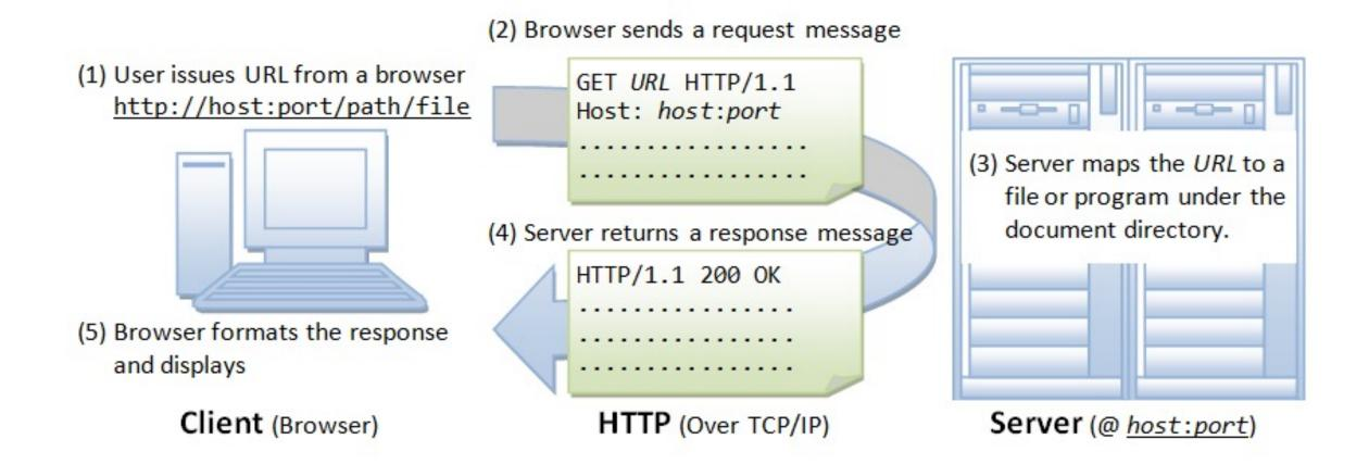
REST generalizes this for machine-to-machine communication
